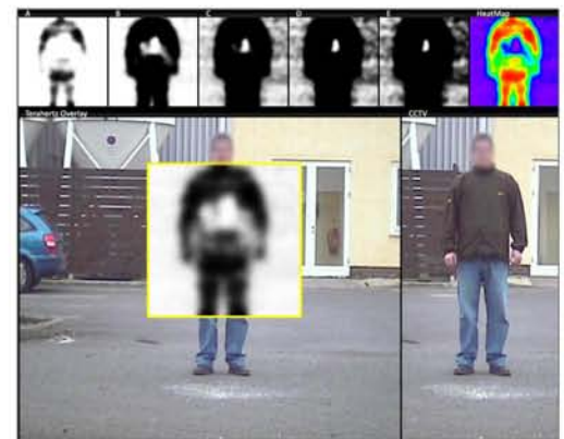
TS5 imagery: In this image the man was concealing an IED at a distance of 12m.
