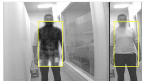
Vertically mounted TS4 - The man was concealing a mobile phone at a distance of 5m
